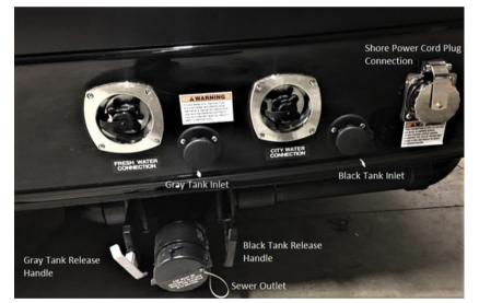
Pull the gray handle - this will dump the gray water tank. Once the tank is empty push the handle back in. The two handles can not be pulled at the same time.
